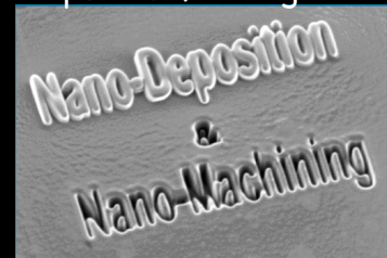
Demonstration by FIB deposition/milling
