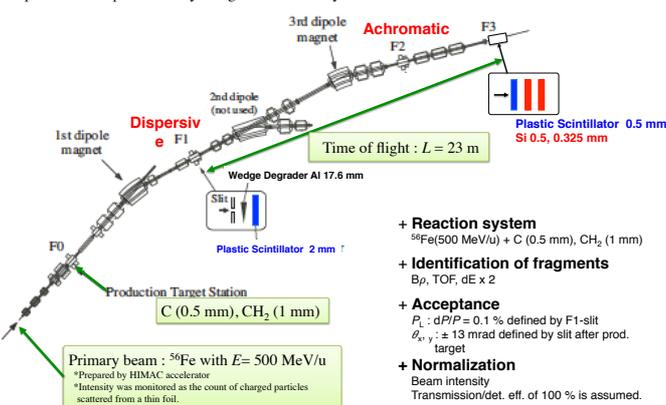
Fig. 4 Secondary beam course SB2 at HIMAC facility
